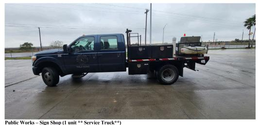
Ford F-350 - 4X4 SuperCrew - 4 doors with Service Body Flat Bed and dual rear wheels
